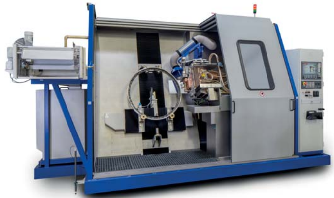
Oblique hardening machine for large bearing races
